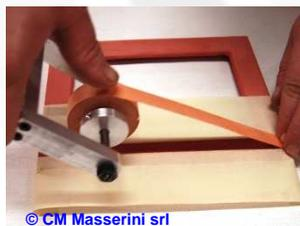
Very useful to gild long and tight sections (gorges of frames). For this fact the rolls are widely used in furniture for thread works.
